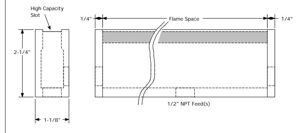
Ensign Model #287 High Capacity T Burner Available in single casting length up to 18" or with welded castings up to 36" 1 or more 1/2" NPT Feed(s) on Bottom, Sides, or Ends Overall Length is 1/2" greater than Flame Space
