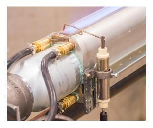
The ERB QuadCool™ Ribbon Burner is a superior choice for Flame Treating surface modification. The innovative SheetFlame design contains no flame ports providing striation-free surface treatments.
