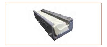
The F-SS-SC is a 12" burner with high temperature, corrosion-resistant alloy side plates and a machined stainless steel baffle plate. The smooth edge of the baffle plate promotes a uniform air/gas flow through the slit orifice, which optimizes the combustion process. The FH-SS-SC is a 7" burner with alloy side and baffle plates. Their corrosion resistance and ability to withstand high temperatures make these two models ideal choices for food applications, such as tortilla chip ovens.
