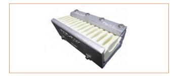
layers surrounding a part. The air-gas mixture travels from the manifold through the body of the burner and is directed onto the refractory through a slit orifice along the length of the burner. The slit orifice design optimizes the life and performance of the burner since it promotes a smooth, consistent flow of gas and is not prone to particulate build-up or clogging as are other designs, such as ported orifices.
