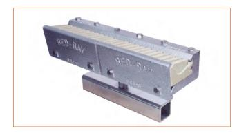
The F Series is a flame impingement gas fired infrared burner. It utilizes an air/gas mixture impinging directly on the finned ceramic refractory surface to produce a high density, radiant flux. The flame heats the refractory to temperatures of 1650°F to 2000°F with a turndown ratio of 4 to 1. The refractory in turn emits thermal energy, achieving approximately 70% convection and 30% infrared. Its maximum output is 4000 Btu/in at 61/2" w.c. mixture pressure.
