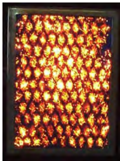
LOW FIRED — Acceptable Operating Condition
