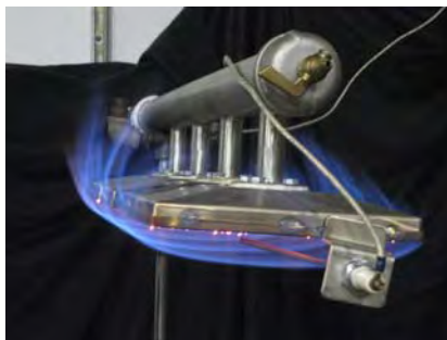
OVER FIRED — UNACCEPTABLE Do Not Operate In This Condition
