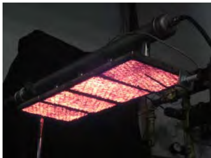
LOW FIRED — Acceptable Operating Condition
