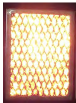
OVER FIRED — UNACCEPTABLE Do Not Operate In This Condition
