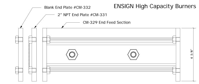
NOTE: End Feed and Bottom Feed sections can be joined togeter to create a burner of any desired length Standard Ribbon slot is 1/2" (nom) Adding the designation W will allow for a Wide Ribbon, or TS for Triple slot
