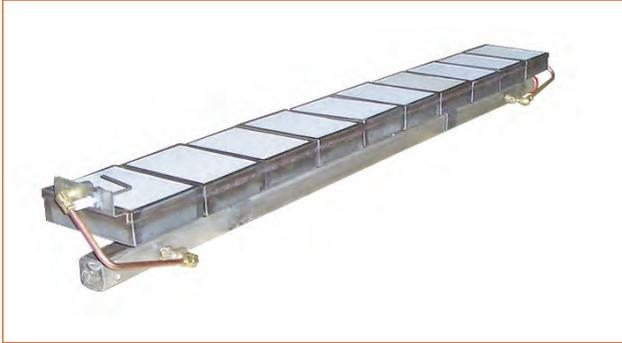
**The MR-86 is a 6" x 8" gas-fired infrared surface combustion burner. Its metal alloy foam emitter and stainless steel body make it an outstanding choice for many food production processes such as browning, pre-cooking or roasting meat. Its high radiance enables rapid searing of meat, allowing the product interior to remain moist. The MR-86 performs well in a wide variety of industrial applications requiring corrosion resistance, high heat flux density and low combustion velocity.**
