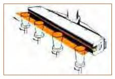
Glassware may be fire-polished or "glazed", to eliminate sharp molded edges that might injure the user. Glazing is frequently performed by fusing the sharp edges while the ware is continuously conveyed through ribbon flames.
