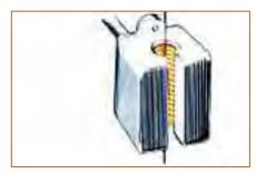
**Wire** is conveniently cured after coating, or otherwise treated, by conveying it vertically through special ribbon burners. Multiple strands are normally heated simultaneously. Burner manifolds are retractable for accessibility.
