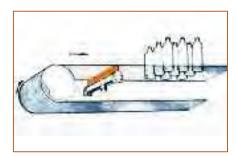
**Conveyors** of ovens, furnaces, and lehrs are preheated to offset effects of cooling during return travel. This practice increases production and reduces thermal shock to previously heated ware.
