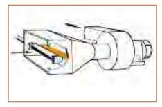
**Air** is heated for many purposes by inducing (or forcing) it over ribbon burners within insulated chambers. Applications include drying, enamel baking, food preparation, curing and similar uses.
