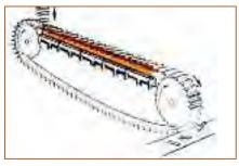
**Parts** of many shapes and materials are handled on conveyors as shown. Fabricated pieces of steel, glass and nonferrous materials are heated for hardening, tempering, annealing or hot forming.
