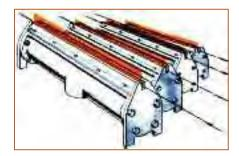
**Filaments** for lamps are preheated ahead of drawing dies, as shown here. Fine sewing threads are singed in multiple strands. Copper alloy wire is heated in this way for annealing.
