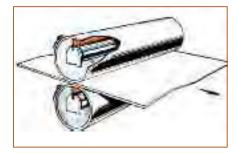
Rolls for calendaring are frequently internally gas fired. The arrangement of ribbon burners provides a suitable means of obtaining uniform lateral heat distribution. Rolls without internal accessibility may be externally fired.
