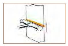
**Webs** are dried, cured or preheated by directing the burner flames against the passing material. Flames are sufficiently uniform to be successfully used for textile singeing. Electrical static is discharged by flame conduction.
