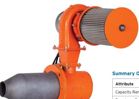
The Selas Superflame™ Pak burner is an innovative adaptation of Selas' proven High Momentum Ceramic Tube (HMCT) low NOx burner. Its compact design features a pre-calibrated linkageless control system, a variable speed fan to conserve energy and low 60 ppm NOx performance at maximum load.
