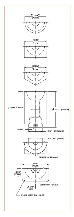
Designed for mounting into vertical refractory walls or panels where 4.5" (114mm) thick wall construction is acceptable, input capacity of the Series 51 tip is adequate, and work temperatures generally do not exceed 1600° to 1800°F (870° to 980°C). All critical metallic parts are fabricated of heat resistant alloy steel.
