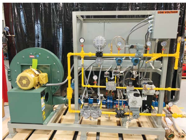
Figure 1: Completed air and gas control system for the 1001 NM burner arrangement.
