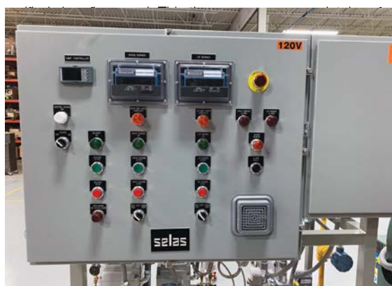
Figure 2: Control panel for the 1001 NM burner arrangement.
