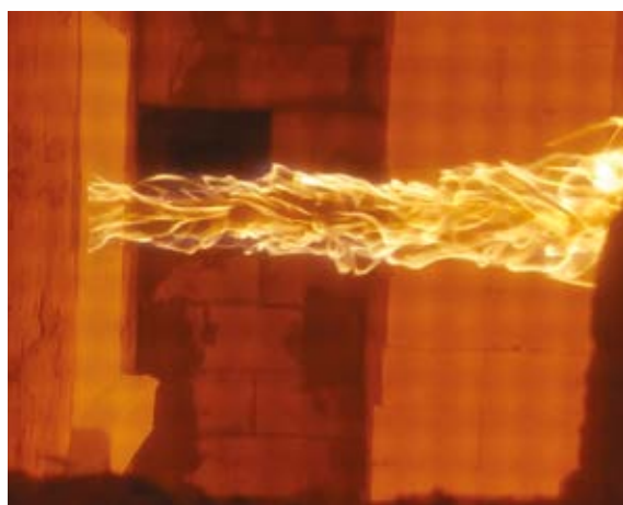
Figure1: The thicker flame root shows strong development for high radiative flux.
