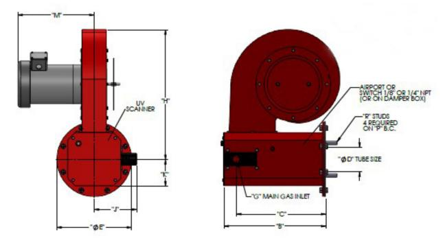
NOTE: All dimensions are in inches  $\pm 1/8$ . Blower mounted sideways on casing w/motor facing mounting plate when no gas train is required. "M" dimension approximate, dependent on motor manufacturer. Dimensions subject to change without notice. Blower may be mounted in other configurations.
