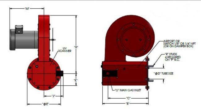
NOTE: All dimensions are in inches ±1/8. Blower mounted sideways on casing w/motor facing mounting plate when no gas train is required. "M" dimension approximate, dependent on motor manufacturer. Dimensions subject to change without notice. Blower may be mounted in other configurations.
