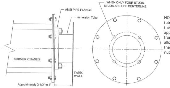
NOTE: Extend the immersion tube out of the tank so that the mounting flange will be approximately 2-1/2" to 3" from the tank wall. This will allow space to reach behind the flange and secure the nuts to the studs.
