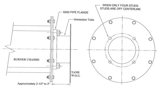
NOTE: Extend the immersion tube out of the tank so that the mounting flange will be approximately 2-1/2" to 3" from the tank wall. This will allow space to reach behind the flange and secure the nuts to the studs.
