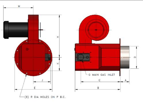
NOTE: All dimensions are in inches +/- 1/8. Blower mounted sideways on casing w/motor facing mounting plate when no gas train is required. 'M' dimensions approximate, dependent on motor manufacturer. Dimensions subject to change without notice. Blower may be mounted in other configurations.
