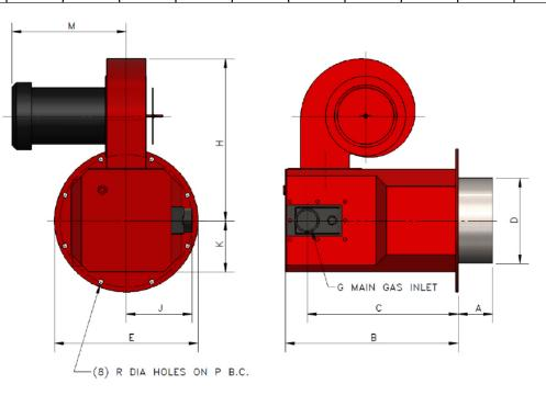
NOTE: All dimensions are in inches +/- 1/8. Blower mounted sideways on casing w/motor facing mounting plate when no gas train is required. 'M' dimensions approximate, dependent on motor manufacturer. Dimensions subject to change without notice. Blower may be mounted in other configurations.
